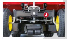
Single block press-forged steel axle
